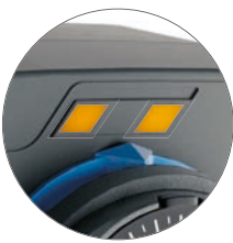
Fig. 14. LEDs in 2- and 3-point actuators
